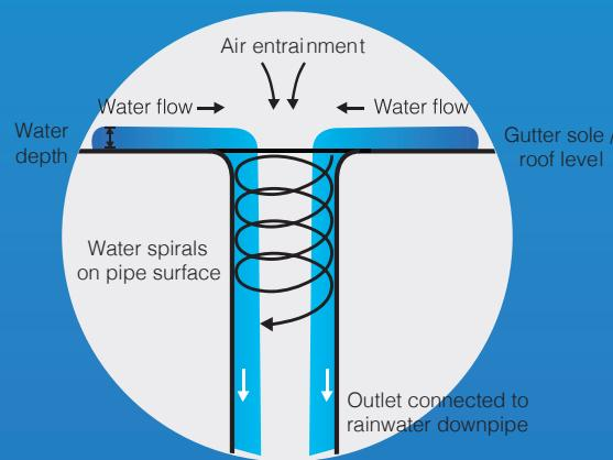
In a traditional drainage system, rainwater on a roof surface flows to the lowest point under gravity. A roof outlet at the gutter low point enables rainwater to connect via a downpipe to the underground drainage system. Both water and air are drawn in and travel through the downpipe in a spiral motion. The capacity of the roof outlet determines how much water can enter the downpipe.
