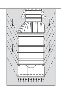
The strategically designed ribs on Ashirvad chambers interlock with the soil to prevent uplift. Engineering calculations that DN 1000 Ashirvad chambers have a safety factor well over 1.8 against buoyancy caused by existing groundwater.
